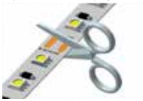
1-1: Cut LED Strip along the cuttable mark
